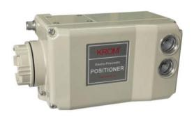
KRA series electro-pneumatic valve positioner is a device that can control the valve opening by receiving the 4-20mA current signal sent by the controller or control system.
